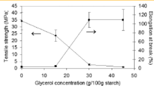
Fig. 1. Effect of the glycerol concentration on tensile strength and elongation at break of cassava starch films
