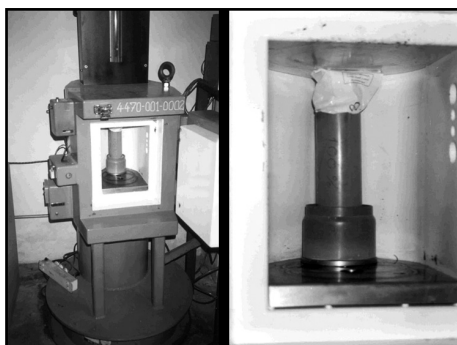
Fig. 2 – Gamma irradiator for irradiation of experimental material for inducing mutations
